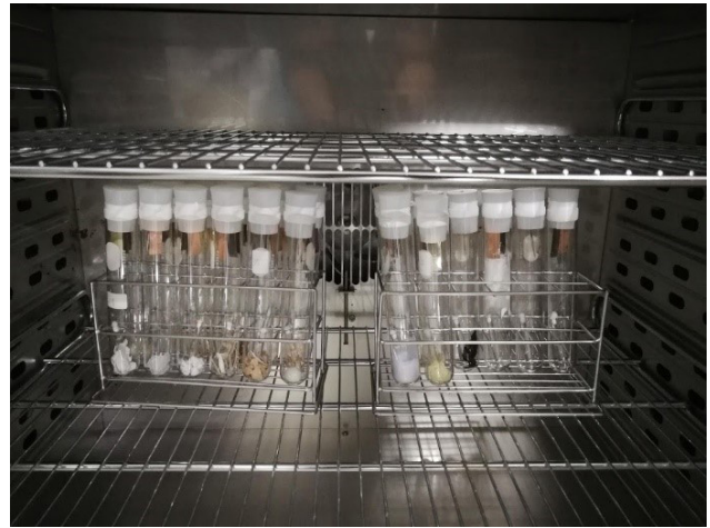
Figure 3. Place filled test tube trays in oven and close door.
